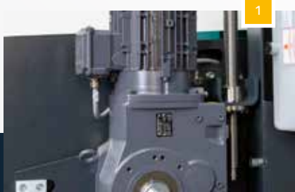
Electronic feed control by ball screw spindle
