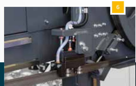
Automatic electronic cutting pressure control
