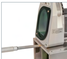
Precise adjustment of the electrode's stick-out.
