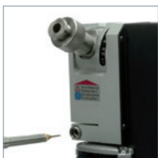
Precise adjustment of the electrode's stick-out.
