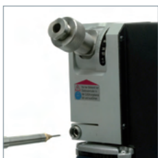
Precise adjustment of the electrode's stick-out.
