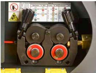
Professional double groove feeding mechanism with 4 rolls
