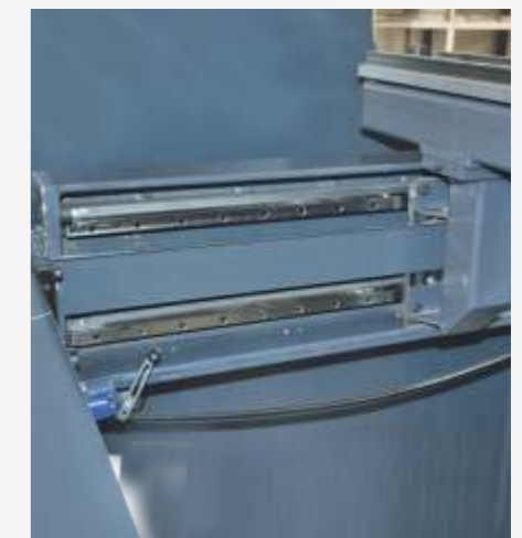
Linear Guided Stronger Back Gauge X Movement
