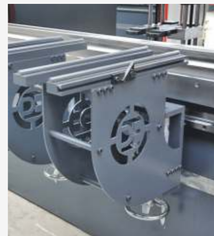
Linear Guided Stronger Front Supports (175 Tons and above machines)
