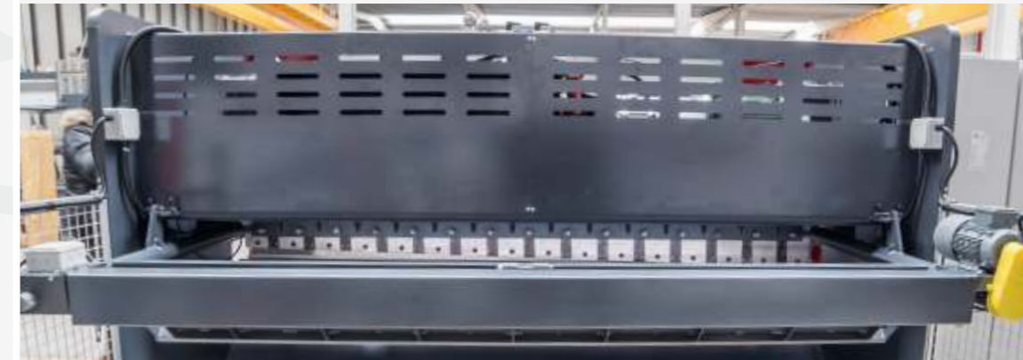
Motorized Back Gauge has \pm 0,1 mm Accuracy
