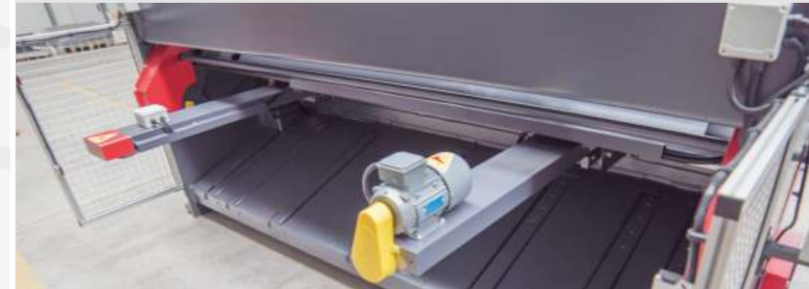
Motorized Back Gauge has \pm 0,1 mm Accuracy
