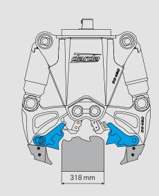
Crusher with additional crushing tips
